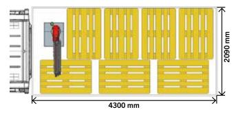
VW Crafter with right **positioned crane (also left position possible),** long wheelbase, simple cabin with load platform: up to max. 7 euro pallets
